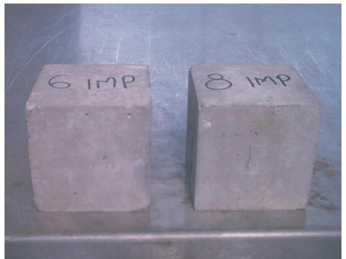
Concrete treated with Evercrete Vetrofluid and subject to 300 freeze-thaw cycles
